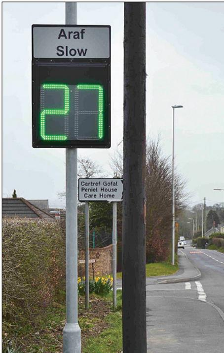
These “driver feedback signs” are traffic calming devices that are proven to give drivers instant feedback as to their speed thereby encouraging a reduced speed where appropriate without the threat of a speeding conviction.
